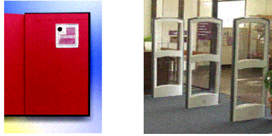
Figure 3.2: On the left, a Checkpoint library RFID tag. On the right, an exit gate.
