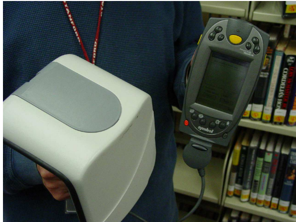
Figure 1.1: Close-up of a library RFID reader and a picture of the reader in use. Pictures courtesy Santa Clara City library.
